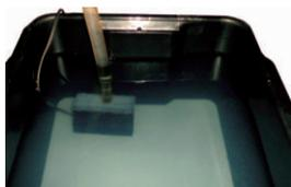
**Fig 1.** This is what can happen to a working nutrient solution when pH is above 7. Calcium, sulfate, copper, iron, manganese and zinc can precipitate on the bottom of the reservoir. In this form and location, they become unavailable to the roots. Further, precipitates can also cause plumbing blockages. To help prevent precipitation, use a nutrient that possesses a high pH buffering capacity.
